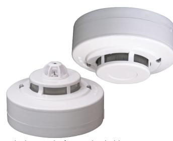
AD-333 series include 2 wire and 4 wire detectors, which provide fast and reliable response to photoelectric smoke and heat  $(135^{\circ}F)$  detection. While the smoke and heat detection circuits operate independently, their outputs being "OR" connected. The detector provide the fire detection performance by acting as a smoke sensor and / or a  $135^{\circ}F$  heat detector at the same location.
